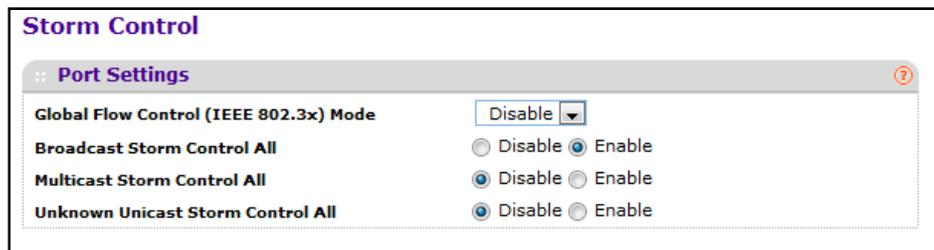
The following four control radio buttons provide an easy way to enable or disable each type of packets be rate-limited on every port in a global fashion. The effective storm control state of each port can be viewed by going to the port configuration page.
