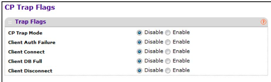
1. **CP Trap Mode** - Displays the captive portal trap mode status. To enable or disable the mode, use the System > SNMP>SNMPv1/v2>Trap Flags page.
