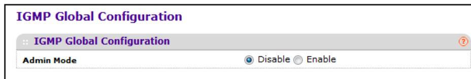
To configure the administrative mode of IGMP on the switch, select the desired option from the **Admin Mode** field. The default is disable. If you change the mode, click **APPLY** to update the switch with the change.
