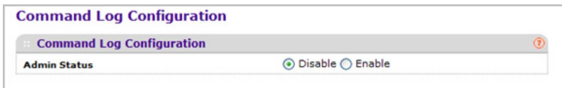
1. Use **Admin Mode** to enable/disable the operation of the CLI Command logging by selecting the corresponding radio button.
